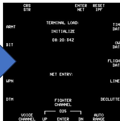
MPCD menu page after JTIDS MODE knob selected to NORM
