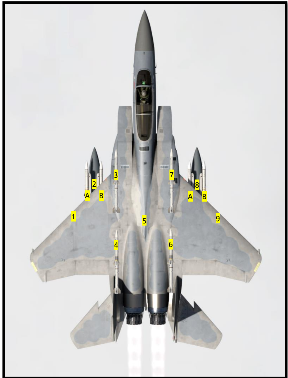
Station Diagram F-15C
